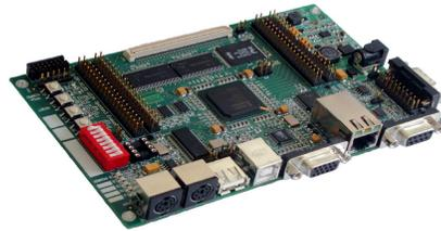
**Fig. 2:** Pender GR-XC3S-1500 Development Board.
