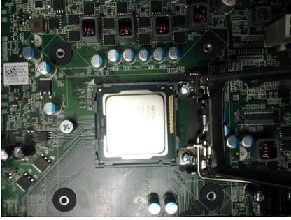
**Fig. 11:** Processor on the Optiplex 7010's motherboard.
